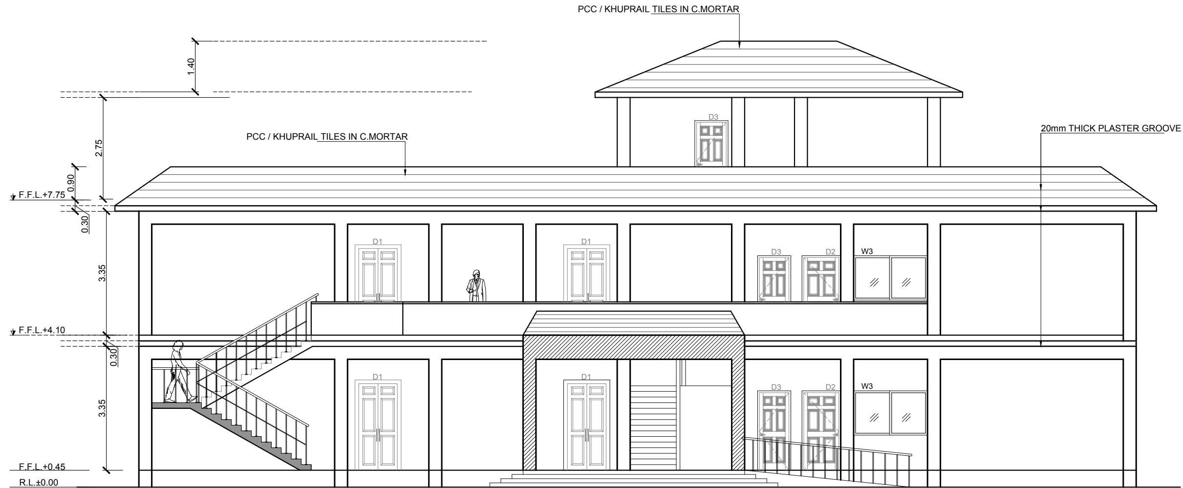
FRONT ELEVATION SCALE A = 1:100
